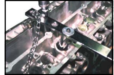
The cotter is adsorbed by the magnet and removed together with the retainer.
