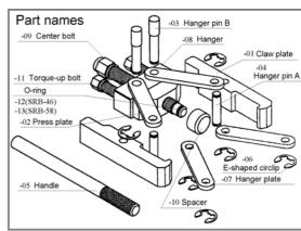
When the center bolt is tightened and then the torque-up bolts are tightened alternately, a larger torque is transmitted by means of the lever action, producing a large output.
