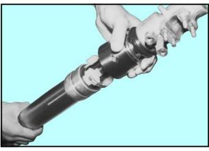
The 3-part attachment is adjusted so that the positions are uniform, and then the attachment is tapped with the detachable sliding hammer to punch the seal into place.
